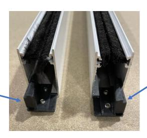
Right hand guide. Wedge on the clip sits to the front of the guide Once they are pushed into the guide insert an allen key into one of the grub screws and slide the clip up the guide to the required position. Note that the top of the handle bar sits under the clip so the opening will be about 40mm lower than the bottom of the clip. See image below
